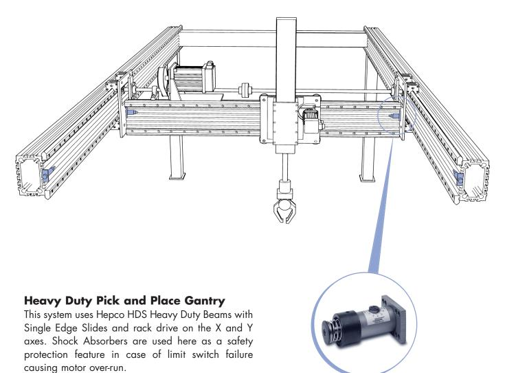
The high value of this gantry set-up means that the small additional investment in shock absorption is well justified to prevent any possibility of damage
